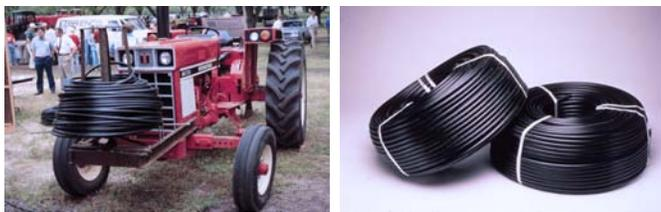
**Figure 3.** Lateral line used in drip irrigation.
