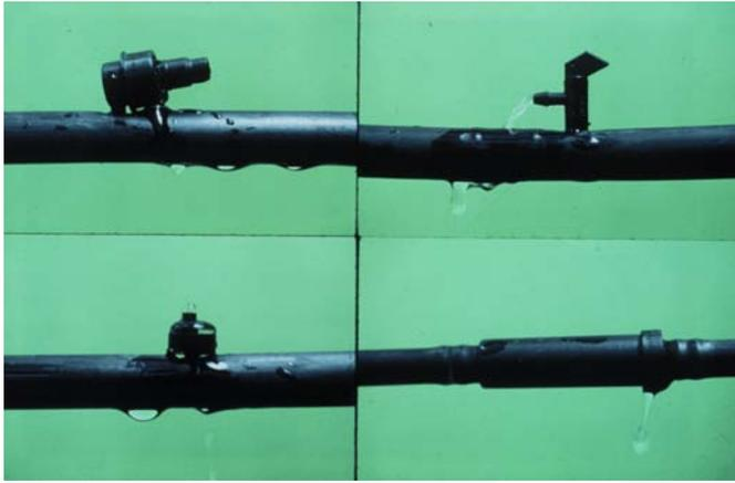
**Figure 1.** Typical emitters for drip irrigation of pecans. Counterclockwise from upper left: Pressure compensating self-flushing emitter; Pressure compensating emitter; Mechanical passageway, in-line, non-flushing emitter; Mechanical passageway manual cleaning emitter.
